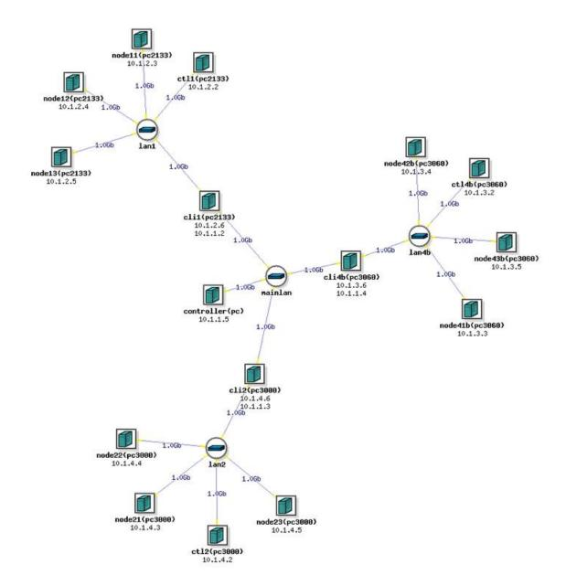
In this example, there are 3 private clouds and they are running in different subnet. By default, all the ip address of virtual machines begins with 10.1.1.1. That means we need to config the IP address of virtual machines, otherwise the nodes in the eucalyptus cannot find these virtual machines even though all the virtual machines are installed successfully.
